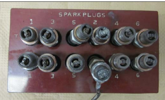
These cylinder #2 spark plugs are packed with melted piston material.
