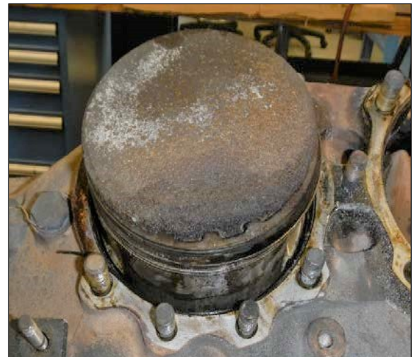
Piston pitting and erosion of the piston face
